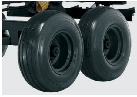
Rodeiro duplo "Sistema Tandem" (DCF-CO 6000 e 8000). Ground wheel with tandem system (DCF-CO 6000 and 8000). Ruedas dobles en los DCF-CO 6000 y 8000 .
